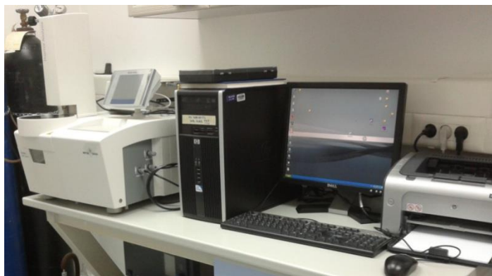
Slika 16. METTLER TOLEDO TGA/DSC System 1
